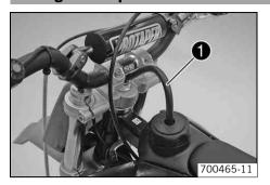
Put the tank cap on and turn it clockwise.
