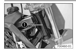
The chassis number • is stamped on right of the steering head.
