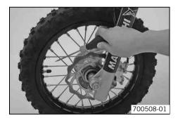
To check spoke tension, tap each spoke with a screwdriver.
