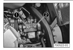
Screw in the idle mixture adjusting screw ② until it stops and then turn to the prescribed basic setting.
