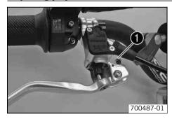
Adjust the play of the handbrake lever with the adjustment screw ①.
