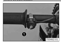
Short circuit button **1** is fitted on the left side of the handlebar.
