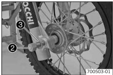
Hold the front wheel and pull out the wheel spindle @ with the washer ③. Take the front wheel out of the fork.
