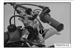
Trottle grip **1** is fitted on the right side of the handlebar.
