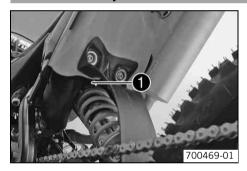
The shock absorber part number  $oldsymbol{0}$  is stamped on the top of the shock absorber above the adjusting ring towards the rear.
