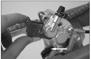
Press both brake shoes into the brake caliper and fix with bolt [2]. Mount the locks [1]. Tighten bolt [2] to 5 Nm (3,7 ft.lb).
