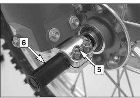
To install the front wheel, lift it into the fork, position and mount the axle shaft. Mount the collar nut [4], tighten the clamping screws [5] on the right fork leg axle passage to prevent the axle shaft from turning and tighten the collar nut to 40 Nm (29,52ft.lb).
