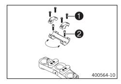
Remove the four screws  $\bullet$ . Remove the handlebar clamp. Remove the handlebar and lay it to one side.
