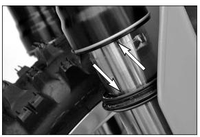
Clean dust-protection bellows, outer tubes, and fork tubes thoroughly, and oil them thoroughly with oil-spray (Motorex Joker 440) or engine oil. Then, push dust-protection bellows into the outer tubes by hand.
