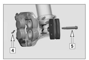
Press both brake shoes and holding spring into the brake caliper and fix with bolt [5]. Tighten bolt to 5 Nm (3.7 ft.lb). Mount the safety device [4]. Align brake shoes, mount front wheel (see chapter: Mounting the front wheel).
