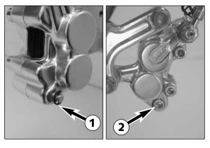
Remove the lock washer • from the screw as well as fixing screw • and take the brake shoes out of the brake caliper. Clean brake caliper thoroughly with compressed air.
