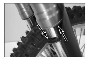
Clean dust-protection bellows, outer tubes, and fork tubes thoroughly, and oil them thoroughly with silicone spray or engine oil. Then, push dust-protection bellows into the outer tubes by hand.
