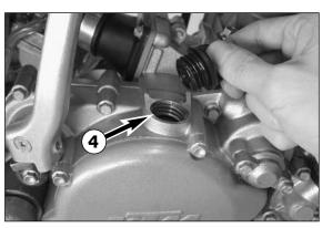
Remove the filler plug @ and add 0.35 I gear oil (e.g. Motorex Topspeed 4T 15W50). Mount the filler plug and check the engine for leaks.
