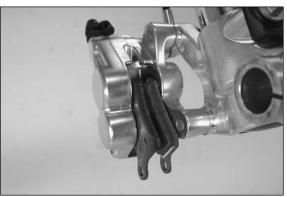
Mount both brake shoes and fasten with the fixing screw. Tighten the fixing screw to 10 Nm. Mount the lock washer. Align the brake shoes, mount the front wheel (see chapter "Mounting the front wheel").
