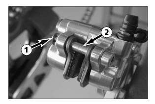
Remove the safety device **1**, knock out the guide pin **2** from the brake caliper with a drift towards the chain wheel and remove the brake pads. Carefully clean the brake caliper with compressed air and check the sleeves of the guide pins for damage.
