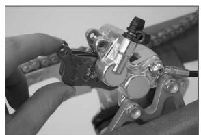
Press both brake shoes into the brake caliper and fix with bolt 2. Mount the locks 1. Tighten bolt 2 to 5 Nm (3,7 ft.lb).
