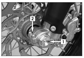
To install the front wheel, lift it into the fork, position and mount the axle shaft [3]. Mount the collar nut [1], tighten the clamping screws [2] on the right fork leg axle passage to prevent the axle shaft from turning and tighten the collar nut to 40 Nm (30ft.lb).
