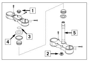
The offset is set to 20 mm in the condition at delivery.
