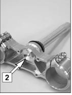
Remove the collar screw from the lower triple clamp and pull out the steering stem. Thoroughly clean all parts. Turn the steering stem 180° and insert it in the triple clamp, tighten the collar screw all the way to the stop. Grease the steering head bearing and sealing elements.
