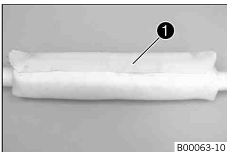
The main silencer is filled with glass fiber yarn ❶.
