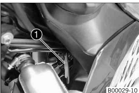
Plug connection ❶ is located in front of the fuel tank on the left side of the frame.
