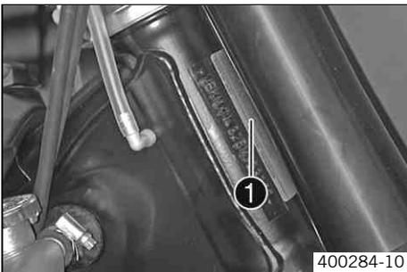
The type label ❶ is fixed to the front of the steering head.
