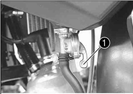
The fuel tap is on the left side of the fuel tank. With tap handle ❶ on the fuel tap, you can open or close the supply of fuel to the carburetor.
