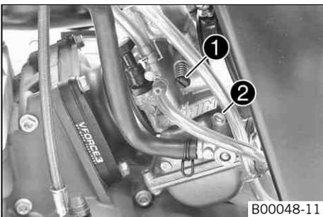
The idle setting of the carburetor has a big influence on the starting behavior, idling stability and the response to opening of the throttle. An engine with a correctly set idle speed is easier to start than if the idle is set wrongly.
