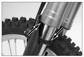
Clean the dust-protection bellows, outer tubes, and fork tubes thoroughly, and oil them thoroughly with silicone spray or engine oil. Then, push the dust-protection bellows into the outer tubes by hand.
