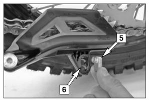
Loosen both screws on the chain guide and pull the chain guide off the swing arm. Turn the chain guide over, press out the retaining nut [5] and insert it in the other hole [6], turning the retaining nut around. Remount the chain guide and tighten the screws.
