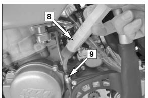
Fill the bleeder syringe [8] with a suitable fluid (see Technical Specifications - Engine). Remove the bleeder screw from the slave cylinder [9] and mount the bleeder syringe.
