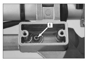
Press oil into the system until the fluid runs out of the hole [1] in the master cylinder without bubbles. Occasionally extract the fluid from the master cylinder reservoir to keep it from overflowing.
