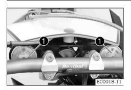
Turn adjusting screws ① clockwise all the way.
