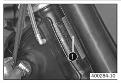
The type label **1** is fixed to the front of the steering head.
