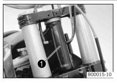
The chassis number  $\bullet$  is stamped on the right side of the steering head.
