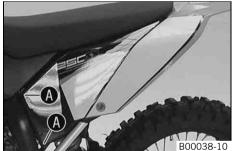
Pull off the air filter box lid in area **()** sideways and remove it toward the front.
