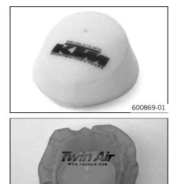
Mount the dust cover for the air filter.
