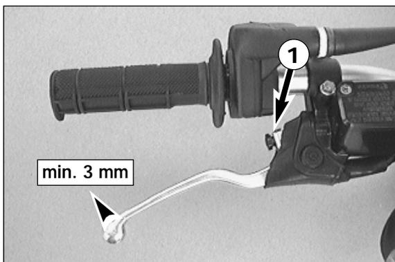
**Adjusting of free travel at the hand brake lever**
