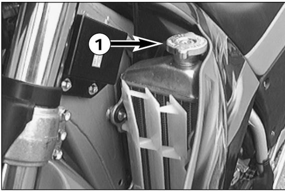
A mixture of 40% antifreeze liquid and 60% water is used as coolant. However, the anti-freeze protection must be at least  $-25^{\circ}\text{C}$  ( $-13^{\circ}\text{F}$ ). This mixture offers antifreeze protection but also good corrosion protection and should therefore not be replaced by pure water.
