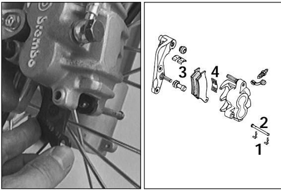
Mount the right brake pad and fix it with the bolt. Mount the left brake pad and insert the bolt until it stops. Mount the clips.
