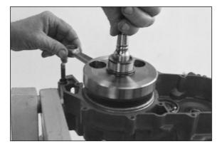
Secure the right-hand housing half in the engine work stand. \_
