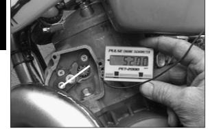
**1.5 Checking the setting of the TVC system** Note: The function of the TVC system is checked with the engine running. This test checks the start of advance and the end of advance.
