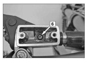
Press oil into the system until the fluid runs out of the hole [6] in the master cylinder without bubbles. Occasionally extract the fluid from the master cylinder reservoir to keep it from overflowing.
