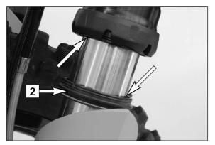
Thoroughly clean the dust boots, slide rings, outer tubes and fork tubes and oil generously with Universal oil spray (Motorex Joker 440) or engine oil. Press the dust boots into the outer tubes by hand. Position the fork protectors, mount the screws and torque to 10 Nm.
