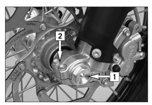
To install the front wheel, lift it into the fork, position and mount the axle shaft [3]. Mount the collar nut [1], tighten the clamping screws [2] on the right fork leg axle passage to prevent the axle shaft from turning and tighten the collar nut to 45 Nm.
