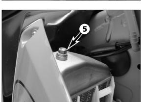
Remove the screw **5** on the right radiator.
