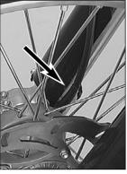
The speedometer shaft must be placed as running along the outside of the fork guard and pas the triple clamp toward the speedometer.
