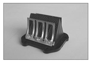
**4.19 Reed valve housing, intake flange** Note: The reed paddles **3** slowly lose their tension during operation, thus reducing the overall performance. Damaged or worn reed paddles must therefore be REPLACED.
