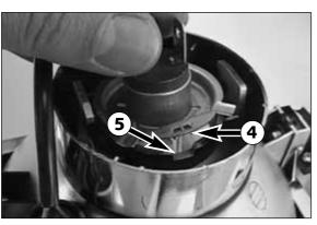
Insert a new bulb such that the noses **④** fit into the recess **⑤**. Do not touch the glass body of the bulb, to keep if free from grease. Mount supporting ring, rubber cap and plug. Position headlight mask with the bottom holders, and fasten it with the rubber bands.
