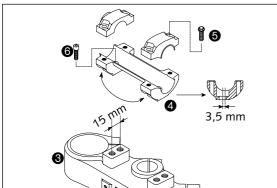
For this purpose, remove screws **③** of the handlebar clamps and screws **③** of the handlebar support. Position handlebar support, and tighten screws **③** to 40 Nm (30 ft.lbs). Mount handlebar and handlebar clamps, and tighten screws **⑤** to 20 Nm (15 ft.lbs). The gap between handlebar support and handlebar clamps is to be of equal size in the front and in the rear.
