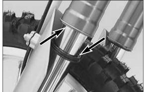
Clean dust-protection bellows, outer tubes, and fork tubes thoroughly, and oil them thoroughly with silicone spray or engine oil. Then, push dust-protection bellows into the outer tubes by hand.
