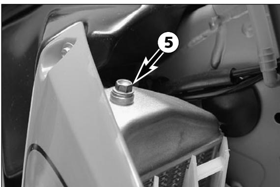
Remove the screw **5** on the right radiator. Now add cooling liquid until it emerges free of bubbles at the right radiator. Then immediately mount the screw so that no more air can enter the right radiator. Top up the left radiator until the coolant can be seen approx. 10 mm (0.4 in) above the radiator fins. Check the coolant level again after a short ride.
