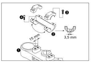
For this purpose, remove screws ③ of the handlebar clamps and screws ④ of the handlebar support. Position the handlebar support, and tighten screws ④ to 40 Nm (30 ft.lbs). Mount the handlebar and handlebar clamps, and tighten screws ⑤ to 20 Nm (15 ft.lbs). The gap between the handlebar support and the handlebar clamps should be the same size in the front and in the rear.
