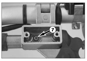
KTM USES BIODEGRADABLE HYDRAULIC OIL FOR THE HYDRAULIC CLUTCH CONTROL. NEVER MIX BIODEGRADABLE HYDRAULIC OILS WITH MINERAL OILS.
