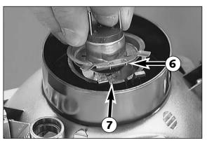
Insert a new lamp such that the noses 6 engage in the recesses 7. When doing so, do not touch the glass body of the lamp so that it remains free from fat. Engage retaining clip, mount rubber cap and connector. If the parking-light lamp is to be replaced, simply insert it in the holder. Reinsert parking-light lamp together with the holder.
