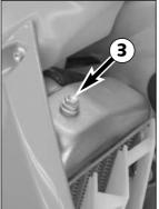
Remove screw ② at the cylinder head. Reinstall it as soon as the cooling liquid emerges free of air bubbles (only for 125/200 engines).
