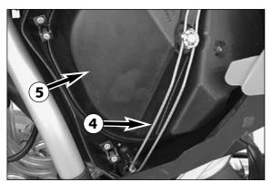
Thoroughly wash the air filter in special cleaning fluid (Motorex Bio Dirt Remover) and allow it to dry well. Only press out the filter, do not wring it out under any circumstances. Oil the dry air filter with a high-grade filter oil (Motorex liquid Bio Power). Also clean the air filter box. Check the carburetor collar for damage and that it is filled correctly.
