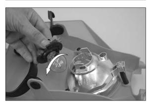
Slightly depress the bulb, turn it approx.  $30^{\circ}$  counterclockwise and pull it out of the socket.
