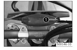
The light switch  $\bullet$  is fitted on the left side of the handlebar.
