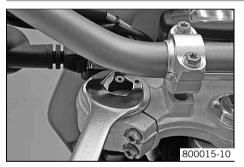
Turn the adjusting screws counterclockwise all the way.
