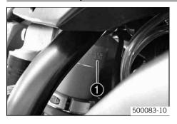
The shock absorber part number  ${\bf 0}$  is stamped on the top of the shock absorber above the adjusting ring on the engine side.
