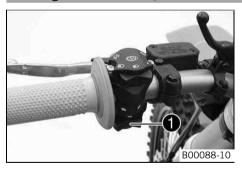
Turn signal switch  $\bullet$  is fitted on the left side of the handlebar.
