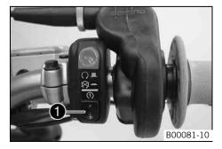
The electric starter button  $\bullet$  is fitted on the right side of the handlebar.
