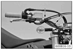
Position the operating elements on the right half of the handlebar.
