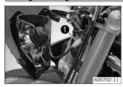
Connect the electric plug connector ①.
