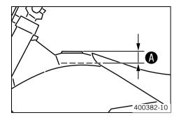
Fill the fuel tank with fuel up to measurement **4**.
