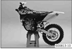
Position the fork legs and tighten the screws of the triple clamp.
