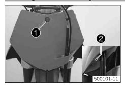
Position the start number plate. Mount and tighten screw • with the spacing sleeve.
