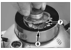
Insert new lamp such that the noses **②** engage the recesses **③** .When doing so, do not touch the glass body of the lamp so that it remains free from fat. Engage retaining clip, mount rubber cap and connector. If the parking-light lamp is to be replaced, simply insert it into the holder. Reinsert parking-light lamp together with holder.
