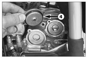
Put the motorcycle on its side and fill the oil filter housings about halfway with engine oil. Insert the long oil filter at the front and the short oil filter at the back of the housing.
