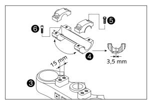
For this purpose, remove screws **6** of the handlebar clamps and screws **6** of the handlebar support. Position handlebar support, and tighten screws **6** to 40 Nm (30 ft.lb). Mount handlebar and handlebar clamps, and tighten screws **6** to 20 Nm (15 ft.lb). The gap between handlebar support and handlebar clamps is to be of equal size in the front and in the rear.
