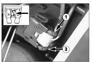
The starter relay also contains a (10 amp) spare fuse **3**.
