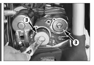
Using circlip pliers, you may now pull the oil-filter inserts 3 out of the housing.
