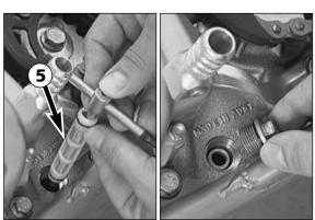
To mount the long oil screen **9**, place it on an approx. 300 mm (12 in) long pin-type key or a similar tool. Insert the pin-type key through the opening into the bore of the opposite engine casing wall. Then, push the oil screen into the engine casing as far as possible. Remove the pin-type key, mount the plug and tighten it to 15 Nm (11 ft.lb).
