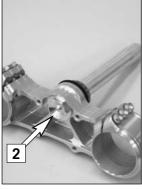
Remove the collar screw from the lower triple clamp and pull out the steering stem. Thoroughly clean all parts. Turn the steering stem 180° and insert it in the triple clamp. Apply Loctite 243 to the thread of the collar screw [2] and turn all the way in.
