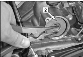
Using circlip pliers, pull the oil-filter insert [2] out of the housing. Clean the oil filter cover, the sealing surface of the O-ring and the engine casing. Check the O-ring of the oil filter covers for damage and, if necessary, replace it
