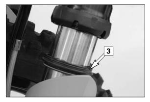
Clean the dust-protection bellows, outer tubes, and fork tubes thoroughly, and oil them thoroughly with Universal oil spray (Motorex Joker 440) or engine oil. Then, push the dust-protection bellows into the outer tubes by hand. Position the fork protector, mount the screws and torque to 10 Nm.
