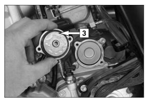
Put the motorcycle on its side and fill the oil filter housing about halfway with engine oil. Fill oil filter with oil, place the oil filter in the filter box. Grease the O-ring  $\hbox{\bf [3]}$  of the oil filter cover and mount the cover. Mount the screws and tighten them to 6 Nm.
