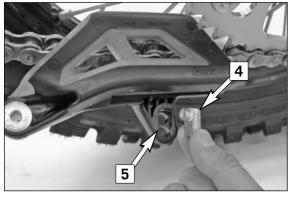
Turn the chain guide over, press out the retaining nut [4] and insert it in the other hole [5], turning the retaining nut around.
