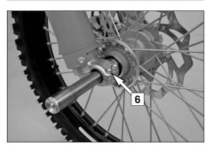
To install the front wheel, lift it into the fork, position and mount the axle shaft. Mount the collar nut [5], tighten the clamping screws [6] on the right fork leg axle passage to prevent the axle shaft from turning and tighten the collar nut to 40 Nm (30ft.lb).
