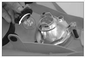
Slightly depress the bulb, turn it approx. 30° counterclockwise and pull it out of the socket.
