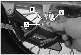
Loosen screw [1] and remove screw [2]. Tilt the chain guide down and insert the collared bush [3] in the corresponding hole. Torque the screws to 10 Nm.
