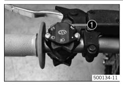
The horn button  $\ensuremath{\bullet}$  is fitted on the left side of the handlebar.
