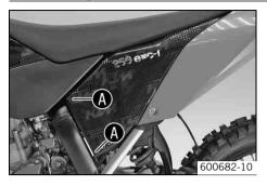
Pull off the air filter box lid in area () to the side and remove to the front.
