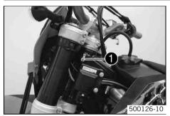
Steering lock **1** is fitted on the left side of the steering head. The steering lock is used to lock the steering. Steering, and therefore riding, is no longer possible.
