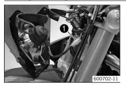
Connect the electric plug connector **①**.
