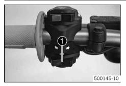
Turn signal  $\bullet$  is fitted on the left side of the handlebar.
