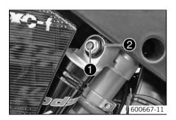
Turn adjusting screw O clockwise with a screwdriver to the last click.
