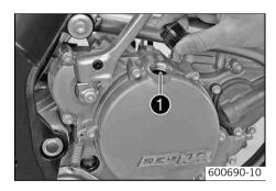
– Remove screw connection  $\ensuremath{0}$  on the clutch cover and fill up with engine oil.
