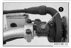
The electric starter button  ${\ensuremath{\bullet}}$  is fitted on the right side of the handlebar.
