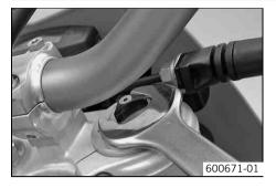
Turn adjusting screws counterclockwise until they stop.
