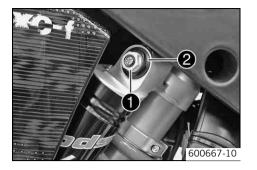
Turn adjusting screw ① clockwise with a ring wrench until it stops.
