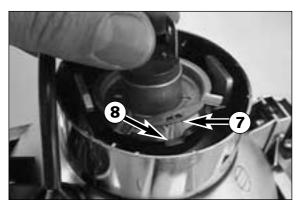
Insert a new bulb such that the noses fit into the recess Do not touch the glass body of the bulb, to keep if free from grease. Mount supporting ring, rubber cap and plug. Position headlight mask with the bottom holders, and fasten it with the rubber bands.
