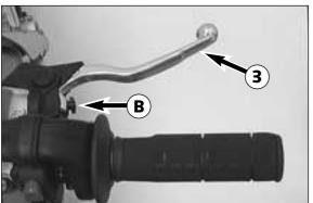
The hand brake lever 3 is mounted on the handle bars on the right and actuates the front wheel brake. The adjusting screw 8 can be used to change the basic position of the hand brake lever (see "Maintenance").
