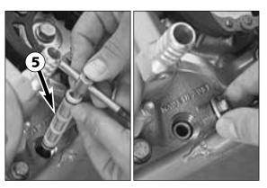
To mount the long oil screen **⑤**, place it on an approx. 300 mm (12 in) long pin-type key or a similar tool. Insert the pin-type key through the opening into the bore of the opposite engine casing wall. Then, push the oil screen into the engine casing as far as possible. Remove the pin-type key, mount the plug and tighten it to 15 Nm (11 ft.lb).
