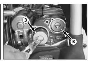
Using circlip pliers, you may now pull the oil-filter inserts 3 out of the housing.
