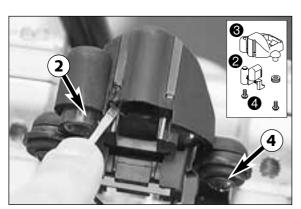
Use a screwdriver to lever the blue speedometer glass 2 downward and out of the speedometer housing **3**. The two noses **4** must be disengaged from the speedometer housing. Remove screws **4**, and take speedometer out of housing.
