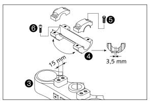
For this purpose, remove screws **6** of the handlebar clamps and screws **6** of the handlebar support. Position handlebar support, and tighten screws **6** to 40 Nm (30 ft.lb). Mount handlebar and handlebar clamps, and tighten screws **6** to 20 Nm (15 ft.lb). The gap between handlebar support and handlebar clamps is to be of equal size in the front and in the rear.
