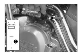
If the inspection glass is heavily soiled (e.g. after a race in muddy terrain), the engine oil level can also be measured with the oil dipstick. For this purpose, unscrew the dipstick and wipe it clean with a cloth. Screw the dipstick back in and screw it out again. If the engine is warm, the oil level should be near the MAX mark (9 (+0mm -5mm) (+0in -0,2in).
