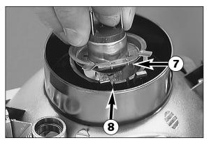
Insert new lamp such that the noses • engage the recesses • .When doing so, do not touch the glass body of the lamp so that it remains free from fat. Engage retaining clip, mount rubber cap and connector. If the parking-light lamp is to be replaced, simply insert it into the holder. Reinsert parking-light lamp together with holder.
