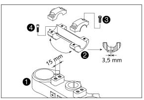
For this purpose, remove screws 3 of the handlebar clamps and screws 4 of the handlebar support. Position handlebar support, and tighten screws 4 to 40 Nm (30 ft.lb). Mount handlebar and handlebar clamps, and tighten screws 5 to 20 Nm (15 ft.lb). The gap between handlebar support and handlebar clamps is to be of equal size in the front and in the rear.
