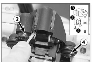
Use a screwdriver to lever the blue speedometer glass 2 downward and out of the speedometer housing **3**. The two noses **4** must be disengaged from the speedometer housing. Remove screws **4**, and take speedometer out of housing.
