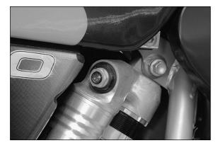
**Damping action during compression of shock absorber (SX)** The shock absorber on the SX models can synchronize the compression damping in the low and high-speed range separately (Dual Compression Control).
