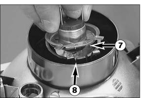
Insert the new lamp such that the noses • engage in the recesses • .When doing so, do not touch the glass body of the lamp so that it remains free from fat. Engage retaining clip, mount rubber cap and connector. If the parking-light lamp is to be replaced, simply insert it in the holder. Reinsert the parking-light lamp together with the holder.
