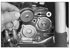
Put the motorcycle on its side and fill the oil filter housings about halfway with engine oil. Fill oil filter with oil, place the long oil filter in the front and the short filter in the back of the filter box.
