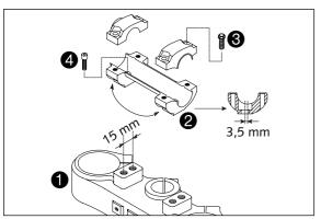
For this purpose, remove screws **3** of the handlebar clamps and screws **4** of the handlebar support. Position the handlebar support, and tighten screws 4 to 40 Nm. Mount handlebar and handlebar clamps, and tighten screws 3 to 20 Nm. The gap between the handlebar support and the handlebar clamps should be the same in the front and in the rear.
