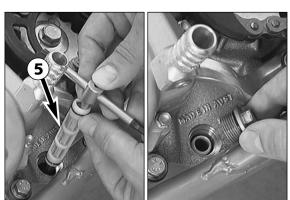
To mount the long oil screen **⑤**, place it on an approx. 300 mm (12 in) long pin-type key or a similar tool. Insert the pin-type key through the opening into the bore of the opposite engine casing wall. Then, push the oil screen into the engine casing as far as possible. Remove the pin-type key, mount the plug and tighten it to 15 Nm.
