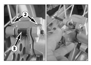
Insert the left brake pad into the brake caliper and secure it with the bolt. Insert the right brake pad and push the bolt ③ into the brake caliper up to the stop. Reattach clips ②.
