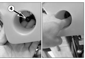
If you pull the choke button 4 out as far as possible, a bore in the carburetor will be opened through which the engine may take in additional fuel. The result is a "fat" fuel-air mixture of the type needed for cold starts. To deactivate the choke, push the choke button back into its basic position.
