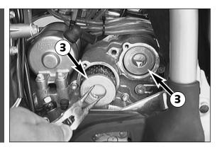
Using circlip pliers, pull the oil-filter inserts ③ out of the housing. Clean the oil filter cover, the sealing surfaces of the O-rings and the engine casing. Check the O-rings of the oil filter covers for damage and, if necessary, replace them.
