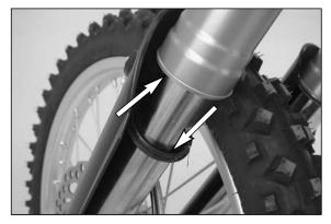
Clean the dust-protection bellows, outer tubes, and fork tubes thoroughly, and oil them thoroughly with Universal oil spray (Motorex Joker 440) or engine oil. Then, push the dust-protection bellows into the outer tubes by hand.
