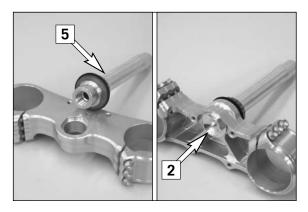
Remove the collar screw from the lower triple clamp and pull out the steering stem. Thoroughly clean all parts. Turn the steering stem  $180^{\circ}$  and insert it in the triple clamp, tighten the collar screw all the way to the stop.
