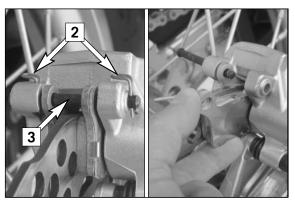
Insert the left brake pad into the brake caliper and secure it with the bolt. Insert the right brake pad and push the bolt [3] into the brake caliper up to the stop. Reattach clips [2].
