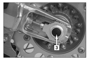
The rear wheel is remounted in the reverse order. Before tightening the collar nut to 80 Nm, push the rear wheel forwards so that the chain tensioners lie on the tension screws.
