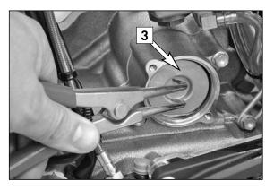
NOTE: The 250-F engine only has one oil filter insert [3].
