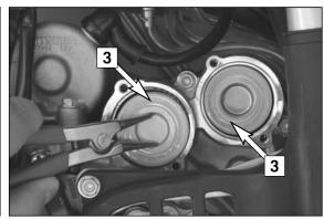
Using circlip pliers, pull the oil-filter inserts [3] out of the housing. Clean the oil filter cover, the sealing surfaces of the O-rings and the engine casing. Check the O-rings of the oil filter covers for damage and, if necessary, replace them.
