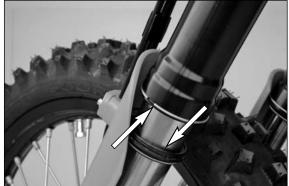
Clean the dust-protection bellows, outer tubes, and fork tubes thoroughly, and oil them thoroughly with Universal oil spray (Motorex Joker 440) or engine oil. Then, push the dust-protection bellows into the outer tubes by hand.
