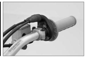
Mount the front wheel fender and tighten the screws to 10 Nm. Mount the hand brake cylinder and tighten the screws to 10 Nm. Mount the starting number plate. Mount the front wheel (see: Dismounting and mounting the front wheel).
