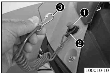
The emergency OFF switch ❶ is mounted on the left in front of the fuel tank. A rip cord is attached to clip ❷. It can be attached to the clothing of the rider by means of carabiner ❸. The emergency OFF switch shuts the engine off if the rider falls off the vehicle.
