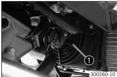
The radiator fan ❶ is located on the radiator under the fuel tank.
