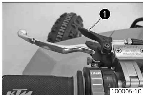
Hot start lever ❶ is fitted on the left side of the handlebar.
