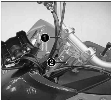
The handlebar position can be adjusted 4-fold by turning the handlebar support ① and the handlebar support ②.
