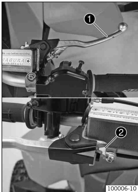
The hand brake lever ❶ is located on the right side of the handlebar and operates the front wheel brakes.
