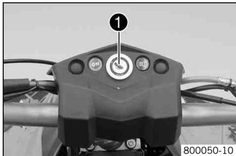
The ignition switch ❶ is located in the instrument support.
