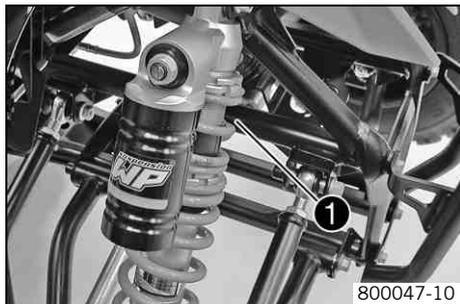
The chassis number ❶ is stamped on the right side of the frame in the vicinity of the upper control arm.
