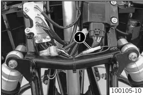
Plug-in connector ❶ is located under the trim at the front on the frame tube.
