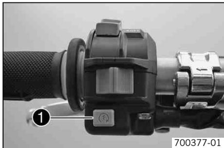
Electric starter button ❶ is fitted on the left side of the handlebar.
