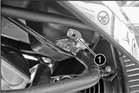
The fuel tap is located on the right side of the fuel tank.
