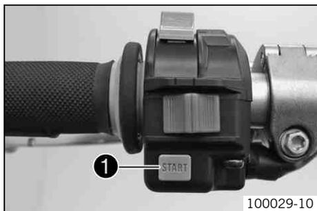
The **START** ❶ electric starter button is fitted on the left side of the handlebar.
