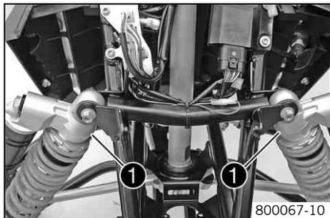
The shock absorber part number ❶ is stamped on the upper part of the shock absorber.
