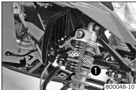
The type label ❶ is located on the frame tube on the right and left in front of the radiator.
