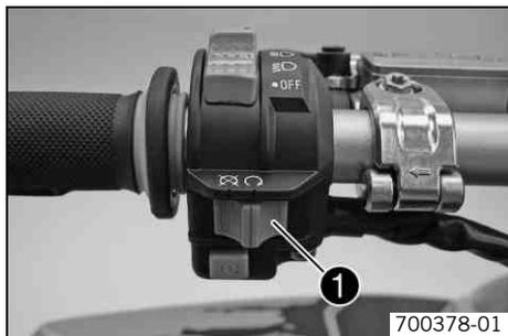
The **ENG. STOP** switch ❶ is fitted on the left side of the handlebar.
