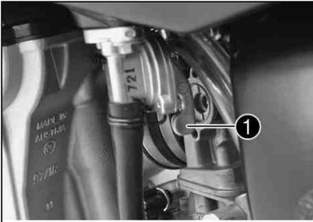
The fuel tap is on the left side of the fuel tank.
