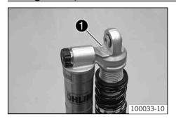
The setting number **1** is stamped into the top of the shock absorber.
