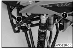
Align the heim joint at right angles to the screws ② and tighten the nut ①.
