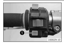
The **START •** electric starter button is fitted on the left side of the handlebar.
