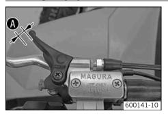
Move the handlebar to the straight-ahead position. Move the reverse gear release lever back and forth slightly to ascertain the play in the Bowden cable .
