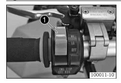
The light switch • is fitted on the left side of the handlebar.
