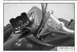
Pull the instrument support off the handlebar and swing it to the side.
