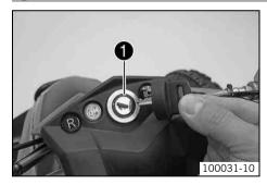
The ignition switch **1** is located in the instrument support.
