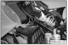
Fill the coolant into the radiator 1.
