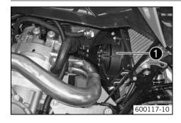
The radiator fan **1** is located on the radiator under the fuel tank.
