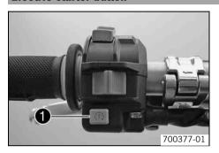
Electric starter button **1** is fitted on the left side of the handlebar.
