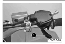
The throttle lever **1** is fitted on the right side of the handlebar. The throttle lever is used to control the engine speed.
