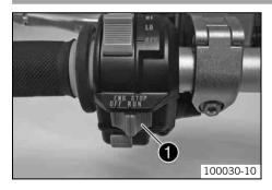
The **ENG. STOP** switch **①** is fitted on the left side of the handlebar.
