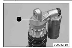
The setting number **1** is stamped into the top of the shock absorber.
