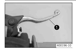
Hand brake lever **1** is located on the right side of the handlebar. The hand brake lever is used to activate the front brake.
