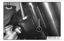
The chassis number **1** is stamped on the steering head on the right.
