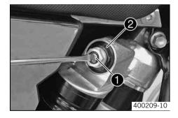
Turn adjusting screw 1 clockwise with a screwdriver up to the last perceptible click.
