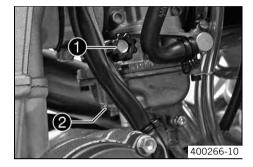
Screw in idle adjusting screw ② until it stops and then to the prescribed basic setting.
