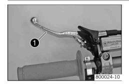
The clutch lever **①** is fitted on the left side of the handlebar. The clutch is hydraulically operated and self-adjusting.
