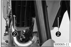
Mount and tighten screws ② with the collar sleeve.
