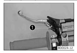
Adjust the basic setting of the clutch lever to your hand size by turning adjusting screw •.
