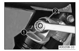
Turn adjusting screw 1 clockwise with a ring wrench until it stops.
