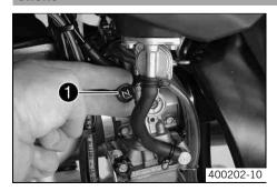
Choke **1** is fitted on the left side of the carburetor.
