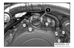
Remove the screw cap • on the clutch cover and fill up with engine oil.
