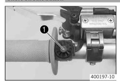
Short circuit button • is fitted on the left side of the handlebar.
