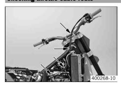
The two throttle cables must run parallel behind the handlebar down to the frame.
