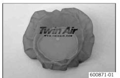
Fit a sand screen device on the air filter.
