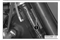
The type label • is fixed to the front of the steering head.
