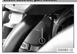
The shock absorber part number **①** is stamped on the top of the shock absorber above the adjusting ring on the engine side.
