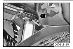
Plug connection • is located in front of the fuel tank on the left side of the frame.
