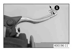
Push the handbrake lever forwards and check the free travel ...
