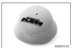
Fit a waterproofing device on the air filter.
