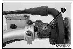
Electric starter button • is fitted on the right side of the handlebar.
