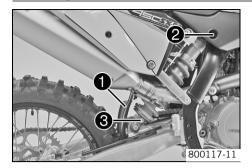
Push splash protector • to the side and position the shock absorber. Mount and tighten screw •.
