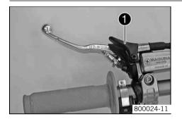
The hot start lever • is fitted on the left side of the handlebar.
