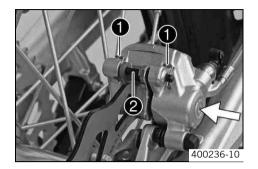
Press the brake caliper by hand onto the brake disc in order to retract the brake piston.
