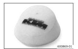
Fit a dust protection device on the air filter.
