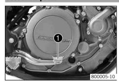
Foot brake pedal **1** is located in front of the right footrest. The foot brake pedal is used to activate the rear brake.
