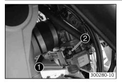
Screw in idle adjusting screw • until it stops and then to the prescribed basic setting.
