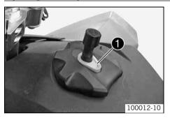
Press release button 1, turn filler cap counterclockwise and lift it free.
