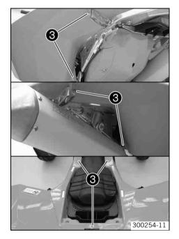
Mount and tighten screws 3.
