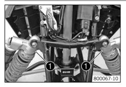
The shock absorber part number **1** is stamped on the upper part of the shock absorber.
