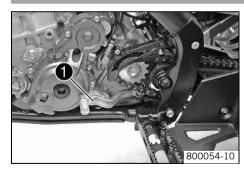
The shift lever • is mounted on the left side of the engine.
