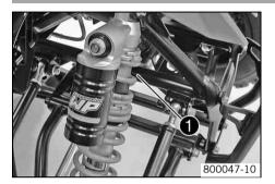
The chassis number lacktriangle is stamped on the right side of the frame in the vicinity of the upper control arm.
