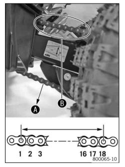
Pull the lower chain section with the specified weight **a**.
