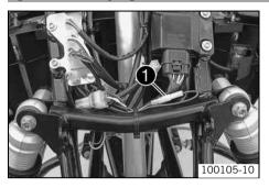
Plug-in connector • is located under the trim at the front on the frame tube.
