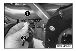
Remove screw • with membrane •.
