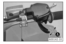
Move the handlebar to the straight-ahead position. Move the throttle lever back and forth slightly to ascertain the play in the gas Bowden cable .
