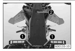
Position the engine guard on the frame bearer. Mount and tighten screws • and •.
