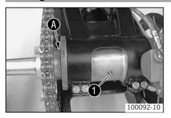
Use a grease gun to fill the rear wheel eccentric element via the grease nipple • until grease emerges from the left shaft seal ring •.
