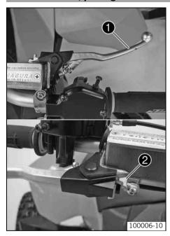
The hand brake lever **1** is located on the right side of the handlebar and operates the front wheel brakes.
