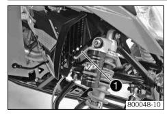
The type label • is located on the frame tube on the right and left in front of the radiator.
