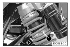
Cross over setting 3 is measured between sliding bushing 1 and the collar of adjusting ring 2.
