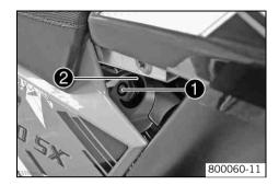
Turn adjusting screw 1 clockwise to the last perceptible click using a screwdriver.
