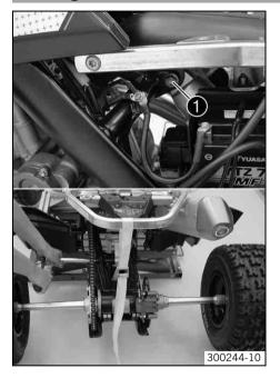
Position the shock absorber in the vehicle with the reservoir on the right. Mount and tighten the top screw ①.
