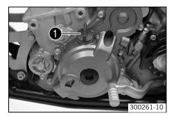
Remove screw cap ● on the clutch cover and fill up with engine oil.
