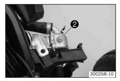
Open screw **②** to bleed the radiator. Tighten the screw when coolant emerges from the opening.
