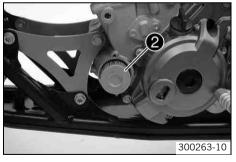
Pull oil filter element ② out of the oil filter case.
