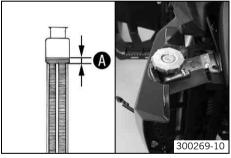
Add coolant to level above the radiator fins.
