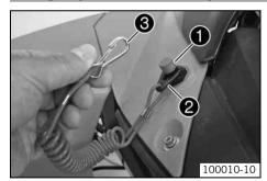
The emergency OFF switch ① is mounted on the left in front of the fuel tank. A rip cord is attached to clip ②. It can be attached to the clothing of the rider by means of carabiner ③. The emergency OFF switch shuts the engine off if the rider falls off the vehicle.
