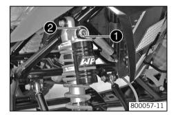
Turn adjusting screw 1 clockwise all the way using a ring wrench.
