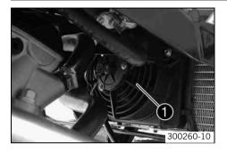
The radiator fan • is located on the radiator under the fuel tank.
