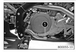
The foot brake pedal • is located in front of the right footrest and operates the rear wheel brake.
