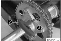
Loosen the screws 1 by four turns.
