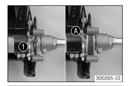
Check that sliding plate • is seated correctly in the brake caliper support and insert the brake linings.
