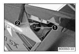
Turn adjusting screw 1 clockwise all the way using a ring wrench.
