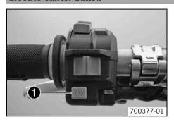
Electric starter button • is fitted on the left side of the handlebar.
