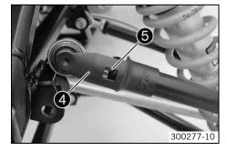
Insert tool 4 in the heim joint and clip onto the A-arm.
