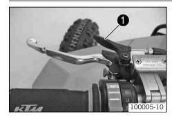
Hot start lever 1 is fitted on the left side of the handlebar.
