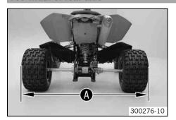
The toe width **4** can be adjusted by installed the spacing sleeve in various ways.
