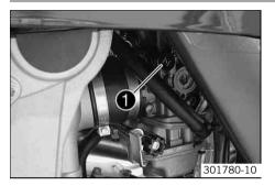
The choke **1** is fitted on the left side of the carburetor.
