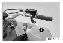
The throttle lever ① is fitted on the right side of the handlebar. The throttle lever is used to control the engine speed.
