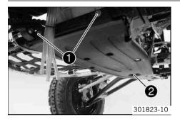
Remove screws **1** and **2**. Remove the engine guard.
