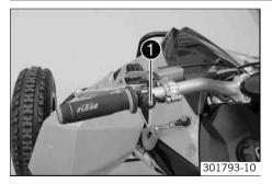
Electric starter button **1** is fitted on the left side of the handlebar.
