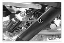
The shock absorber part number **1** is stamped on the upper part of the shock absorber.
