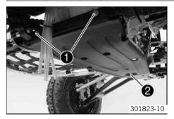
Position the engine guard on the frame bearer. Mount and tighten screws ① and ②.
