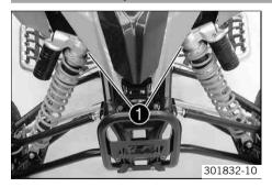
The shock absorber part number  $\bullet$  is stamped on the upper part of the shock absorber.
