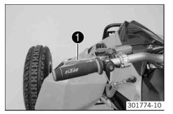
The clutch lever **1** is fitted on the left side of the handlebar.
