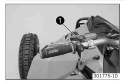
Hot start lever 1 is fitted on the left side of the handlebar.
