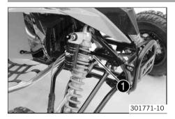
The chassis number  ${\bf 0}$  is stamped on the right side of the frame in the vicinity of the upper control arm.
