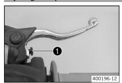
Adjust the basic setting of the handbrake lever to your hand size by turning adjusting screw •.
