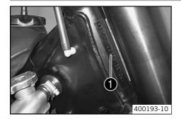
The chassis number **1** is stamped on the right side of the steering head tube.
