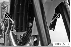
Pull both spoilers to the side of the radiator bracket 3 and take the fuel tank away upwards.
