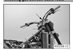
The two gas Bowden cables must run parallel behind the handlebar down to the frame. They must be routed directly on the frame above the tank bearing to the carburetor.
