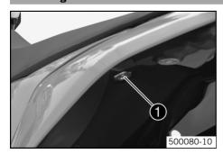
Remove screw ①. Lift up the seat at the rear, pull it back and then remove from above.
