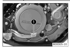
Foot brake pedal • is located in front of the right footrest. The foot brake pedal is used to activate the rear brake.
