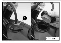
Press release button •, turn filler cap counterclockwise and lift it free.
