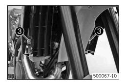
Pull both spoilers to the side of the radiator bracket 3 and take the fuel tank away upward.
