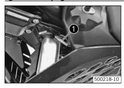
Plug connection • is located in front of the fuel tank on the left side of the frame.
