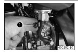
Choke **1** is fitted on the left side of the carburetor.
