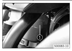
The shock absorber part number lacktriangle is stamped on the top of the shock absorber above the adjusting ring on the engine side.
