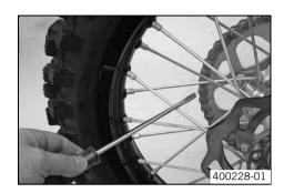
To check spoke tension, tap each spoke with a screwdriver.
