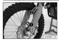
Position the fork protection on the left fork leg. Mount and tighten screws ①.
