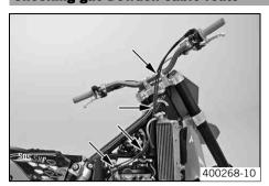
The two gas Bowden cables must run parallel behind the handlebar down to the frame. They must be routed directly on the frame above the tank bearing to the carburetor.
