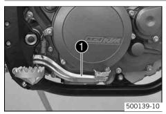
Foot brake pedal **①** is located in front of the right footrest. The foot brake pedal is used to activate the rear brake.
