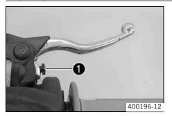
Adjust the free travel of the handbrake lever with the adjustment screw **1**.
