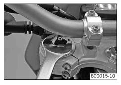
Turn adjusting screws counterclockwise until they stop.
