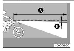
On a light-colored wall behind a horizontal area, make a mark as high as the center of the headlight.
