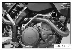
Kickstarter **1** is fitted on the right of the engine. The engine can be started with either the kickstarter or the electric starter. The upper part of the kickstarter can be swung out.
