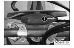
The light switch **1** is fitted on the left side of the handlebar.
