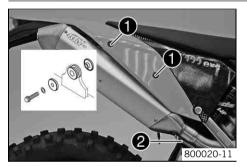
Mount the main silencer. Mount and tighten screws ①.
