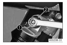
Turn the adjusting screw **1** clockwise with a ring wrench until it stops.
