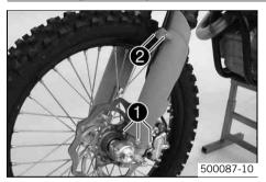
Position the fork protection on the left fork leg. Mount and tighten screws ①.
