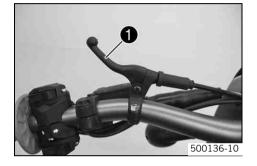
Choke **1** is fitted on the left side of the carburetor.
