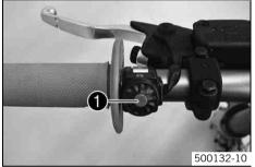
The short circuit button **1** is fitted on the left side of the handlebar.
