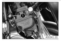
Screw in the idle adjusting screw **2** until it stops and then to the prescribed basic setting.
