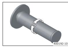
Move the handlebar to the straight-ahead position. Move the throttle grip backwards and forwards to ascertain the play in the gas Bowden cable.
