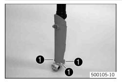
Position the fork protection on the left fork leg. Mount and tighten screws ●. Guideline
