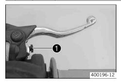
Adjust the basic setting of the handbrake lever to your hand size by turning adjusting screw **1**.
