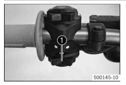
Flasher switch **1** is fitted on the left side of the handlebar.
