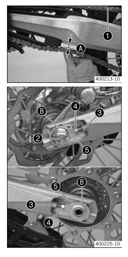
Push the chain at the end of the chain sliding component upwards to measure chain tension A.
