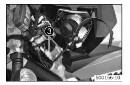
Pull out the electric plug connector  $\ensuremath{\mathfrak{G}}$  and remove the headlight mask with the headlight.
