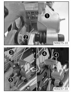
Check that leaf spring ● in the brake caliper and sliding plate ❷ in the brake caliper support are seated correctly.
