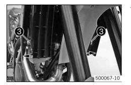
Pull both spoilers to the side of the radiator bracket  $\ensuremath{\mathfrak{S}}$  and take the fuel tank away upwards.
