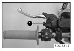
Adjust the basic setting of the clutch lever to your hand size by turning adjusting screw  $\bullet$ .
