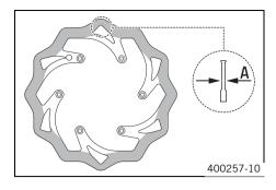
Check the thickness of the front and rear brake discs at several places on the disc to see if it conforms to measurement **(3**).
