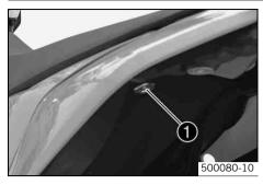
Remove screw **1**. Lift up the seat at the rear, pull it back and then remove from above.
