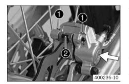
Press the brake caliper by hand on to the brake disc in order to press back the brake piston.
