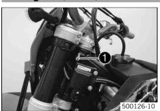
Steering lock ① is fitted on the left side of the steering head. The steering lock is used to lock the steering. Steering, and therefore riding, is no longer possible.
