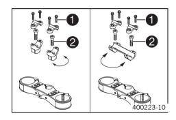
Remove the four screws  ${\bf 0}.$  Remove the handlebar clamp. Remove the handlebar and lay it to one side.
