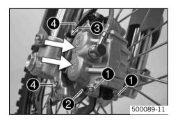
Press the brake caliper by hand on to the brake disc in order to press back the brake pistons.
