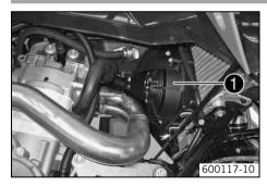
The radiator fan • is located on the radiator under the fuel tank.
