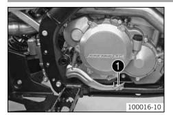
The foot brake lever **①** is located in front of the right footrest. The foot brake lever activates the brakes of all four wheels.
