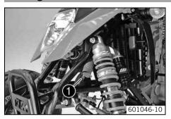
The steering lock **1** is fitted on the steering column.
