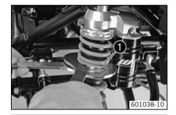
Measure the cross over setting 3 between sliding bushing 2 and the collar of adjusting ring 3.
