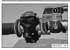
The electric starter button • is fitted on the left side of the handlebar.
