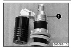
The shock absorber part number **1** is stamped on the top part of the shock absorber.
