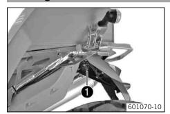
Pull the release hook • back. Lift up the seat at the rear, pull it back and then remove from above.
