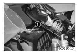
Fill the coolant into the radiator ①.
