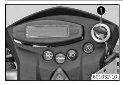
The ignition switch **1** is located to the right of the speedometer.
