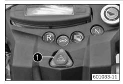
The hazard warning flasher switch **1** is fitted centrally below the indicator lamps. The hazard warning flasher is used to indicate emergency situations.
