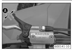
Move the handlebar to the straight-ahead position. Move the reverse gear release lever back and forth slightly to ascertain the play in the Bowden cable <sup>(a)</sup>.
