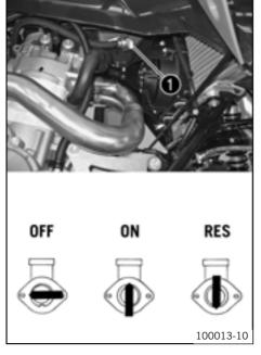
The fuel tap is located on the right side of the fuel tank.
