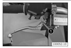
Adjust the basic setting of the handbrake lever to your hand size by turning adjusting screw **①**.
