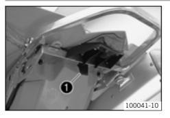
Pull the release hook ① back. Lift up the seat at the rear, pull it back and then remove from above.
