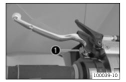
Adjust the basic setting of the clutch lever to your hand size by turning adjusting screw ①.
