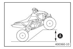
Position the vehicle as shown and secure it against rolling away. The height difference
