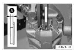
Check the brake linings of both front brake calipers for minimum thickness 0.
