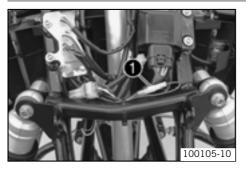
The plug-in connector **①** is located under the trim at the front on the frame tube. **Possible states**
