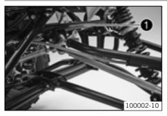
The chassis number **1** is stamped on the right side of the frame in the vicinity of the upper control arm.
