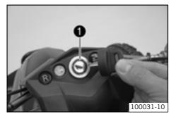
The ignition switch **1** is located on the instrument support.
