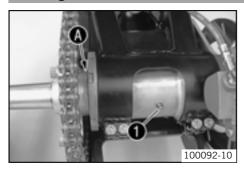
Use a grease gun to fill the rear wheel eccentric element via the grease nipple
