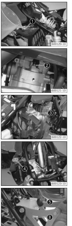
Fill the coolant into the radiator ①.
