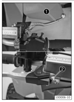
The hand brake lever  $\bullet$  is located on the right side of the handlebar and operates the front brakes.
