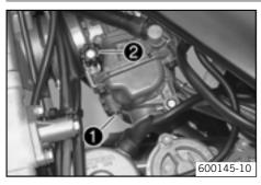
Screw in the idle adjusting screw **1** until it stops and then to the prescribed basic setting.
