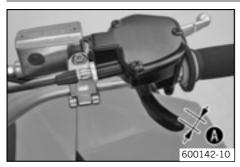
Move the handlebar to the straight-ahead position. Move the throttle lever back and \_ forth slightly to ascertain the play in the gas Bowden cable  $\boldsymbol{0}$ . Specification
