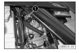
The choke knob **1** is fitted on the left side of the carburetor. Activating the choke function frees an opening through which the engine can draw extra fuel. This gives a richer fuel-air mixture, which is needed for a cold start.
