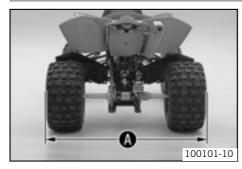
The toe width () can be adjusted by installed the spacing sleeve in various ways.
