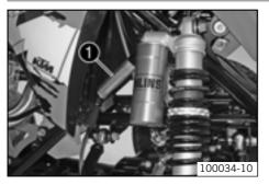
The type label  $\bullet$  is located on the frame tube on the right in front of the radiator.
