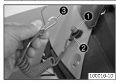
The emergency OFF switch  $\bullet$  is mounted on the left in front of the fuel tank. A rip cord is attached to the clip @. It can be attached to the clothing of the rider by means of a carabiner $\bullet$ .
