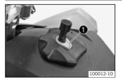
Press release button ①, turn filler cap counterclockwise and lift it free.
