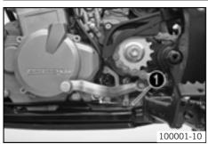
The engine number  $\bullet$  is stamped on the left side of the engine under the engine sprocket.
