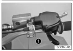
The throttle lever **1** is fitted on the right side of the handlebar. The throttle lever is used to control the engine speed.
