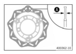
Check the thickness of the front and rear brake discs at several places on the disc to see if it conforms to measurement **()**.
