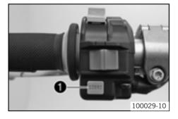
The **START O** electric starter button is fitted on the left side of the handlebar.
