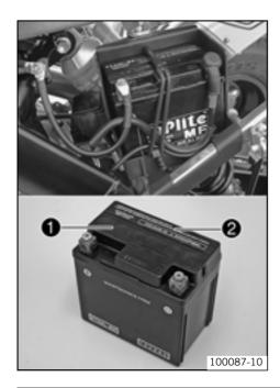
Connect the battery charger to the battery. Switch on the battery charger.
