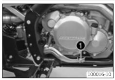
The foot brake pedal  $\bullet$  is located in front of the right footrest and operates the rear wheel brake.
