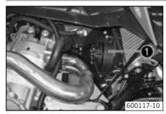
The radiator fan  $\ensuremath{\bullet}$  is located on the radiator under the fuel tank.
