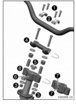
Pull the instrument support off the handlebar and swing it to the side.
