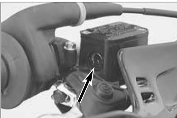
**Checking of brake fluid level - front brake**
