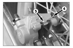
Slide left brake pad into the brake caliper and fix it with the pin. Slide in the right brake pad and knock the bolt in as far as it will go. Mount safety device  $\mathbf{\Phi}$ .
