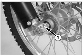
To install the front wheel, lift it into the fork, position and mount the axle shaft. Mount the collar nut **2**, tighten the clamping screws **0** on the right fork leg axle passage to prevent the axle shaft from turning and tighten the collar nut to 40 Nm (30ft.lb).
