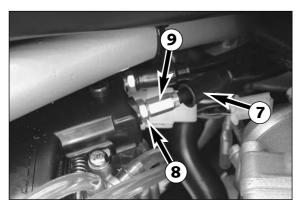
To adjust the throttle cable, push back the protection cover **②**, loosen the counter nut **③** and turn the adjusting screw **④** as required. Turning the adjusting screw counterclockwise will reduce the backlash, turning the adjusting screw clockwise will increase the backlash.
