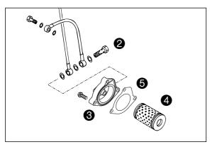
Place the new oil filter **3** on the connection in the oil filter cover and mount together with a new seal **5**. Tighten the 3 screws in the filter cover to 5 Nm. Tighten the hollow screw with seals and tighten to 15 Nm. Finally, start the engine and check the oil system for leakage.
