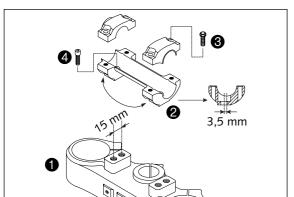
For this purpose, remove screws **3** of the handlebar clamps and screws **4** of the handlebar support. Position handlebar support, and tighten screws **4** to 40 Nm (30 ft.lbs). Mount handlebar and handlebar clamps, and tighten screws **3** to 20 Nm (15 ft.lbs). The gap between handlebar support and handlebar clamps is to be of equal size in the front and in the rear.
