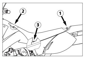
When installing the seat, be sure to insert the rear portion of the seat into the metal clasp **3**.
