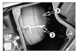
Remove the air filter from the filter holder and wash thoroughly in special cleaning fluid. Motorex offers environmentally-friendly products for professional oil filter maintenance (Motorex Bio Dirt Remover + Motorex Liquid Bio Power). Press out the water from the air filter but do not wring and allow the filter to dry. Lubricate the dry air filter thoroughly with highgrade filter oil, rubbing to coat the entire filter surface.
