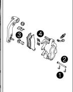
Mount the right brake pad and fix it with the bolt. Mount the left brake pad and insert the bolt until it stops. Mount the clips.
