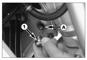
Fill 0.6 liters (0.16 US gallons) of engine oil into the can and remove the plug • next to the steering head. Introduce the plastic hose into the vent hole •, (see page 30) and fill 0.6 liters (0.16 US gallons) of engine oil into the frame's front tube. Remove plastic hose, start engine, and let it idle (approx. 20 seconds) until oil escapes at the hole •. As soon as oil begins to leak out, switch off the engine, mount the plug and gasket and tighten to 25 Nm.
