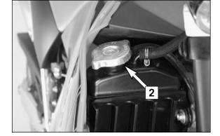
A mixture of 50% anti freeze liquid and 50% water is used as coolant. However, the anti-freeze protection must be at least  $-25^{\circ}$  C ( $-13^{\circ}$  F). This mixture offers anti-freeze protection but also good corrosion protection and should therefore not be replaced by pure water.
