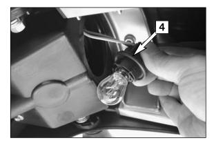
Turn the lamp socket [4] approximately 30° counterclockwise and pull it out of the tail light housing.
