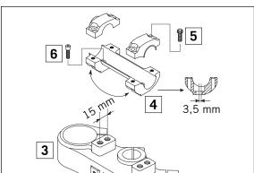
For this purpose, remove screws **[5]** of the handlebar clamps and screws **[6]** of the handlebar support. Position handlebar support, and tighten screws **[6]** to 40 Nm (30 ft.lbs). Mount handlebar and handlebar clamps, and tighten screws **[5]** to 20 Nm (15 ft.lbs). The gap between handlebar support and handlebar clamps is to be of equal size in the front and in the rear.
