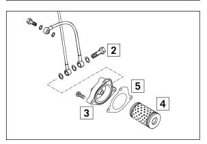
Place the new oil filter [4] on the connection in the oil filter cover and mount together with a new seal [5]. Tighten the 3 screws in the filter cover to 5 Nm. Tighten the hollow screw with seals and tighten to 15 Nm. Finally, start the engine and check the oil system for leakage.
