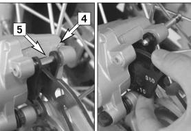
Slide left brake pad into the brake caliper and fix it with the pin. Slide in the right brake pad and knock the bolt in as far as it will go. Mount safety device [4].
