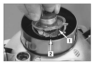
Insert the new lamp such that the noses [1] engage in the recesses [2]. When doing so, do not touch the glass body of the lamp so that it remains free from fat. Engage retaining clip, mount rubber cap and connector. If the parking-light lamp is to be replaced, simply insert it in the holder. Reinsert the parking-light lamp together with the holder.
