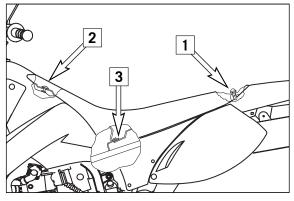
When installing the seat, be sure to insert the rear portion of the seat into the metal clasp [3].
