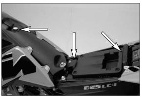
When you mount the seat, make sure the retaining brackets are fastened to the seat.
