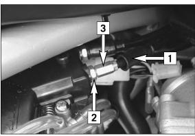
To adjust the throttle cable, push back the protection cover [1], loosen the counter nut [2] and turn the adjusting screw [3] as required. Turning the adjusting screw counterclockwise will reduce the backlash, turning the adjusting screw clockwise will increase the backlash.
