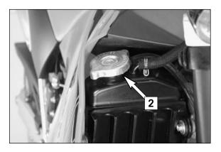
A mixture of 50% anti freeze liquid and 50% distilled water is used as coolant. However, the anti-freeze protection must be at least -25° C (-13° F). This mixture offers anti-freeze protection but also good corrosion protection and should therefore not be replaced by pure water.
