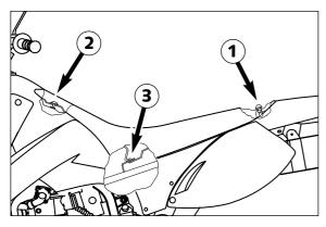
When installing the seat, be sure to insert the rear portion of the seat into the metal clasp  $\odot$ .
