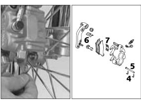
Mount the right brake pad and fix it with the bolt. Mount the left brake pad and insert the bolt until it stops. Mount the clips.
