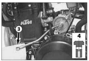
It is necessary to bleed the micro filter so that all friction areas can be quickly supplied with engine oil. To do this, fill with oil and remove the jet screw from the oil line on the clutch cover. Start the engine and close off the oil filler hole on the clutch cover with a rag. Allow the engine to run at idle until oil runs out of the oil line Turn the engine off. Install seal rings and the jet screw. Torque the jet screw to 10 Nm (7 ft.lb) and check for leaks.
