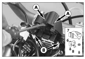
Use a screwdriver to lever the blue speedometer glass  $\odot$  downward and out of the speedometer housing  $\odot$ . The two noses  $\odot$  must be disengaged from the speedometer housing. Remove screws  $\odot$ , and take speedometer out of housing.
