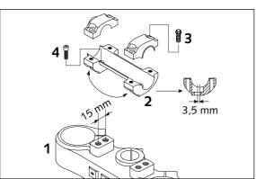
For this purpose, remove screws ③ of the handlebar clamps and screws ④ of the handlebar support. Position handlebar support, and tighten screws ④ to 40 Nm (30 ft.lbs). Mount handlebar and handlebar clamps, and tighten screws ⑤ to 20 Nm (15 ft.lbs). The gap between handlebar support and handlebar clamps is to be of equal size in the front and in the rear.
