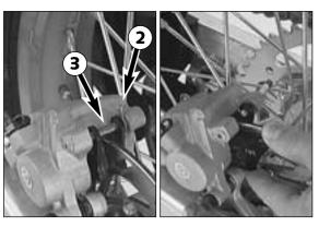
Slide left brake pad into the brake caliper and fix it with the pin. Slide in the right brake pad and knock the bolt in as far as it will go. Mount safety device ②.
