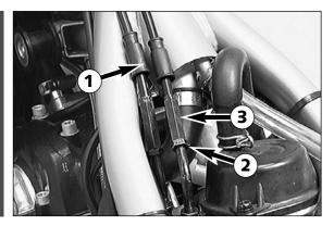
If a correction is necessary, start by removing the tank. Slide back the protection cover lacktriangle. To set the backlash, loosen the counter nut  $\it 2$  and turn the adjusting screw  $\it 3$  accordingly. Then, fasten the counter nut and slide the protection cover back on.
