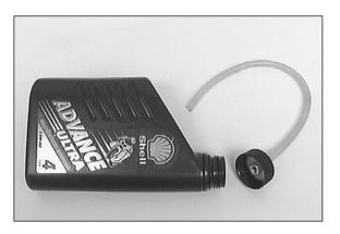
To facilitate bleeding of the oil system, we have added a hose connection piece and a plastic hose to the set of tools. Take an empty oil can (1 liter) and drill a 7 mm-diameter hole into the lid. Screw the hose connection piece into the lid from the outside, and secure it from the inside with the M8 hexagon nut.
