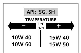
**Engine oil**Use only synthetic oil brands, which meet quality requirements (ShellAdvance Ultra 4) of API-classes SG or SH (informations on bottles) or higher.
