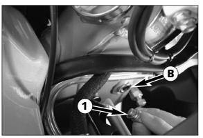
Fill 0.6 liters of engine oil into the can and remove the plug ① next to the steering head. Introduce the plastic hose into the vent hole ③, (see page 30) and fill 0.6 liters of engine oil into the frame's front tube. Remove plastic hose, start engine, and let it idle (approx. 20 seconds) until oil escapes at the hole ③. As soon as oil starts to escape, turn off the engine, and mount the plug together with the gasket.
