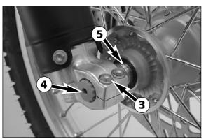
Before mounting, check if the left and the right 6 distance bushing are correctly positioned in the shaft seal rings. Extremely soiled distance bushings should be removed, cleaned and regreased.
