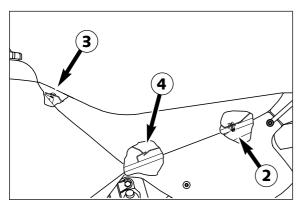
To install the seat, hook the seat into the oval-head screw, set the rear portion down on the frame, and slide it forward. If necessary, press down on the front area of the seat so that the seat catches on the retaining bracket **4**. Insert and tighten the collar screw.
