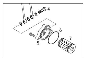
Check the O-ring () for damage. O-rings need not be replaced unless damaged. Press the O-ring into the groove of the filter cover. Fit new oil filter () with rubber gasket on the fitting in oil filter cover and mount cover with filter. Mount three screws and tighten with 5 Nm (4 ft.lb). Mount hollow screw with seal rings and tighten with 15 Nm (11 ft.lb). Start engine and check oil system for leakage.
