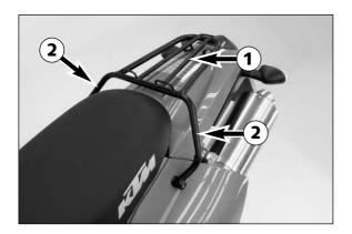
**Baggage carrier / Grips**The baggage carrier may be loaded with up to 10 kg. The two lateral hoops serve as handles for the passenger
