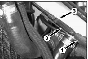
Push the choke lever all the way to the front and slide the protecting cap from the adjusting part 2.
