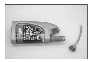
To facilitate bleeding of the oil system, we have added a hose connection piece and a plastic hose to the set of tools. Take an empty oil can (1 liter) and drill a 7 mm-diameter hole into the lid. Screw the hose connection piece into the lid from the outside, and secure it from the inside with the M8 hexagon nut.
