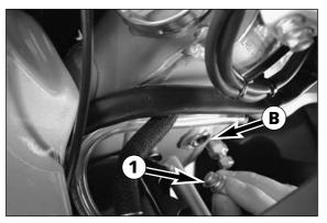
Fill 0.6 liters of engine oil into the can and remove the plug ① next to the steering head. Introduce the plastic hose into the vent hole ③, (see page 30) and fill 0.6 liters of engine oil into the frame's front tube. Remove plastic hose, start engine, and let it idle (approx. 20 seconds) until oil escapes at the hole ③. As soon as oil starts to escape, turn off the engine, and mount the plug together with the gasket and tighten to 25Nm.
