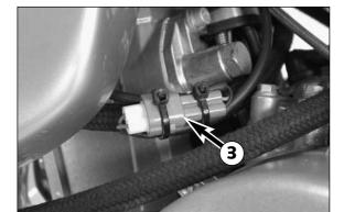
Mount the tank carefully. Mount the insulating disk, steel disk and collar nut and tighten. Connect the fuel lines and open the fuel cocks. Connect the plug and socket connector for the gasoline level sensor and fix to the fuel lines with cable clips.
