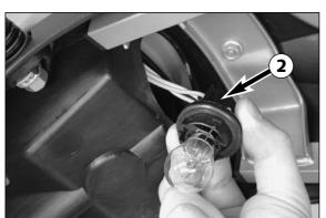
Turn the lamp socket **2** approximately 30° counterclockwise and pull it out of the tail light housing.
