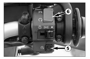
The emergency off switch 6 is provided for emergency situations and should not be used to switch off the engine.
