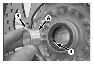
Before remounting the front wheel, clean and grease the shaft seal rings and the bearing surface of the distance bushings and mount the distance bushings (wide distance bushing in the left shaft seal ring). Slightly push back the brake pads with a screwdriver. Position the front wheel against the brake disks according to the direction of travel (see arrow ).
